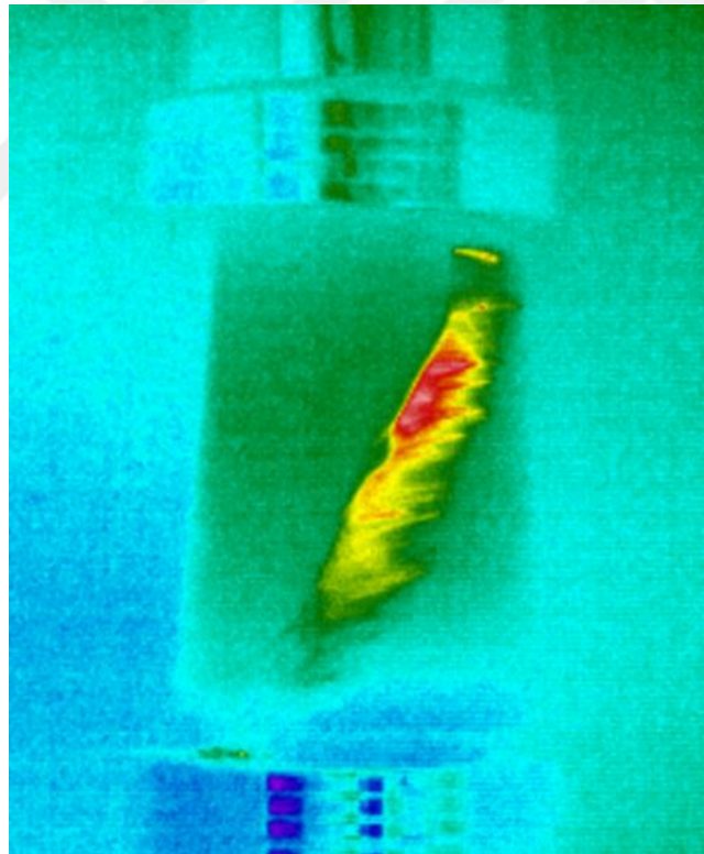
Figure B.20. Failure plane detection of the NLUCS-37 sample by the thermal camera
