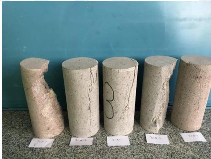
Figure 3.8. Andesite specimens with 75 mm diameter after test
