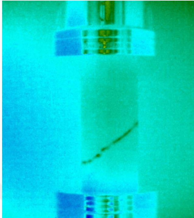
Figure B.29. Failure plane detection of the NLUCS-62 sample by the thermal camera
