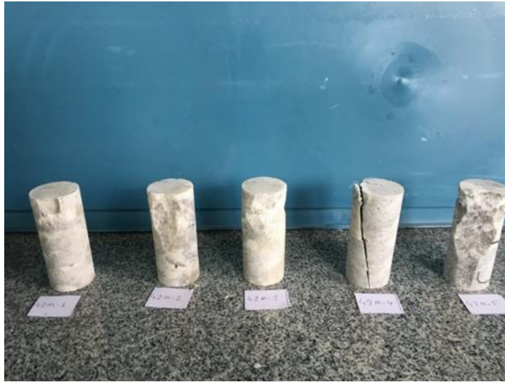
Figure 3.22. Marble specimens with 42 mm diameter after test
