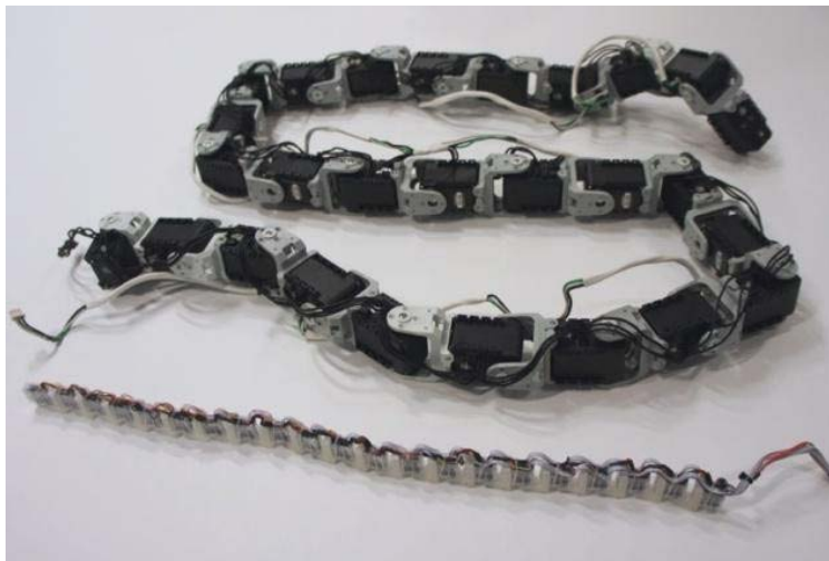
Figure 3.13 : LineFORM consisting of tiny servo-motors (URL-8).
