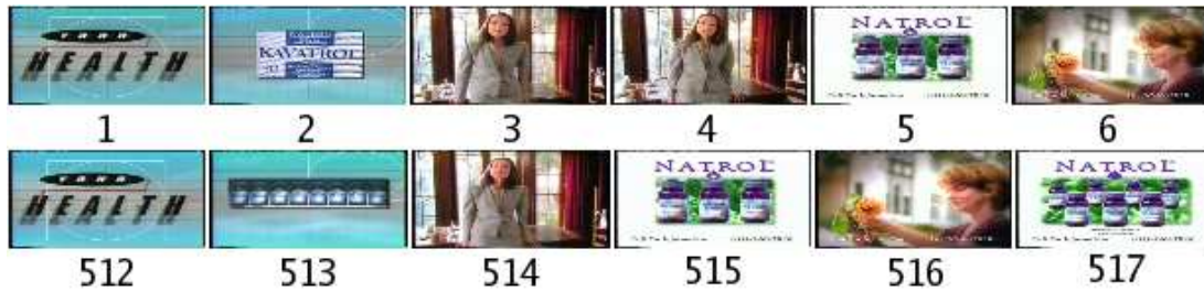
Figure 3.6: An example of unequal Period Constraint from TRECVID dataset. First row represents real sequence and second row represents repeating sequence. Numbers below frames are frames numbers in time domain. Although first frame in first row satisfies Period Constraint with 511 frames, last frame in the same row satisfies with 510 frames.
