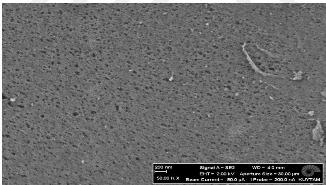
Figure 3.8: Porous structure of alginate aerogel inside the PET nonwoven composite
