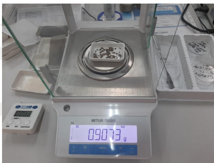
Figure 3.6 Olive residue particles weighted for slow pyrolysis experiment
