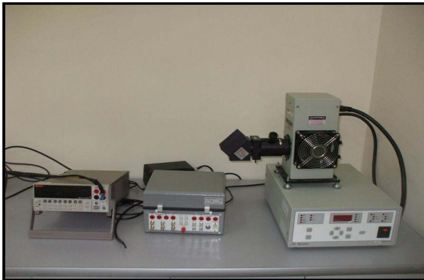
Figure 3.9a. Current-voltage measurement system with Keithley 2400 sourcemeter and Oriel solar simulator
