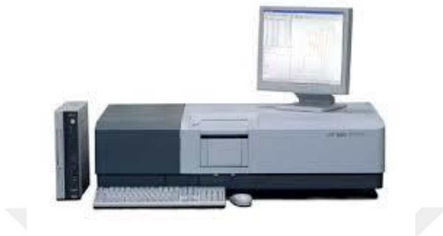
Figure 3.10. Shimadzu 3600 Uv-vis-nir spectrophotometer
