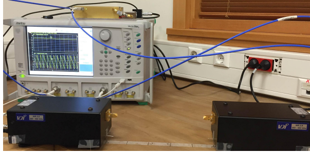
Figure 2.2: THz Band channel measurement setup.
