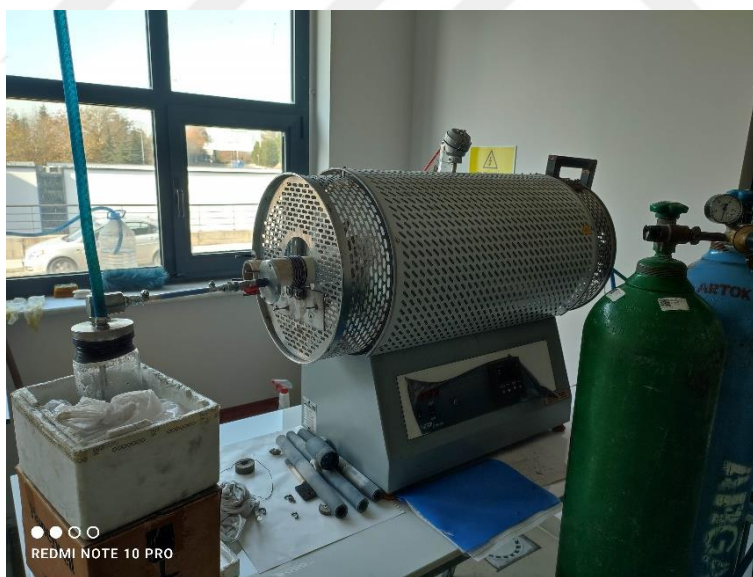
Figure 3.9. The DTM modified rotary furnace.
