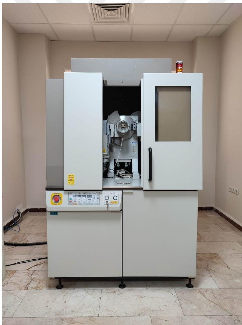
Figure 3.12. Rigaku D/MAX/2200-PC device used in the characterization of powders
