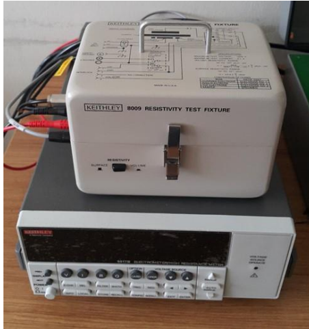
Figure 3.18 An electrometer and a resistivity chamber for the resistivity measurements
