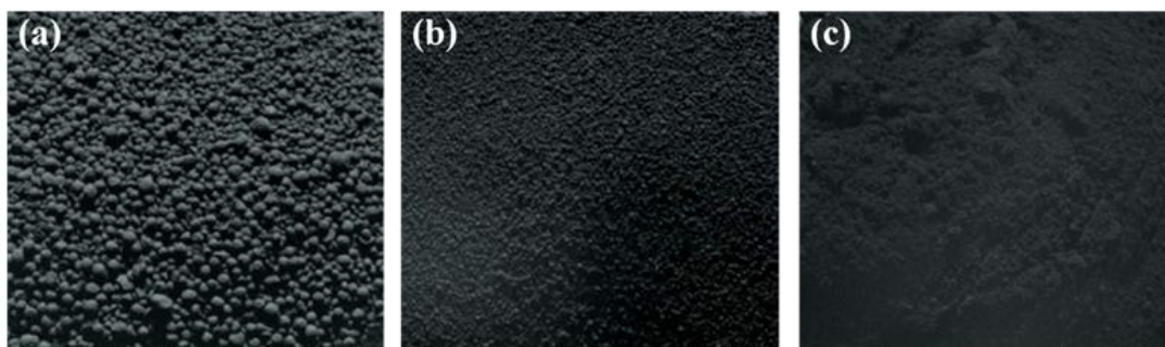
Figure 2.7 Carbon black in the form of a) wet pelletized, b) dry pelletized, c) powder [144]
