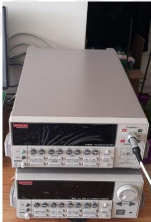
Figure 3.19 Current source and Nanovoltmeter used for resistance measurement
