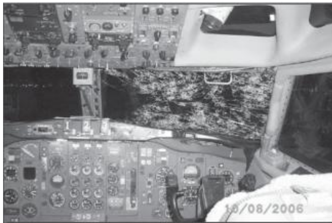
Figure 2.2: Hail damage to a cockpit window [31].
