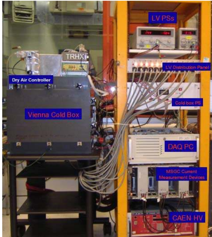
Figure 4.9. Module Long-Term Testing System and its components.
