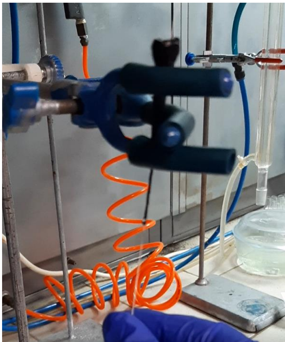
Figure 3.10. Coating process for yarn-shaped anodes
