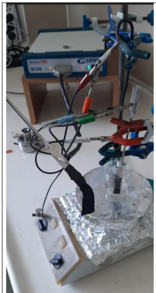
Figure 3.17. Measurement of electrochemical properties of electrodes using 3-electrode method
