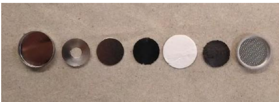
Figure 3.22. Picture of battery components before assembly. b. Diagram showing the order of assembly.
