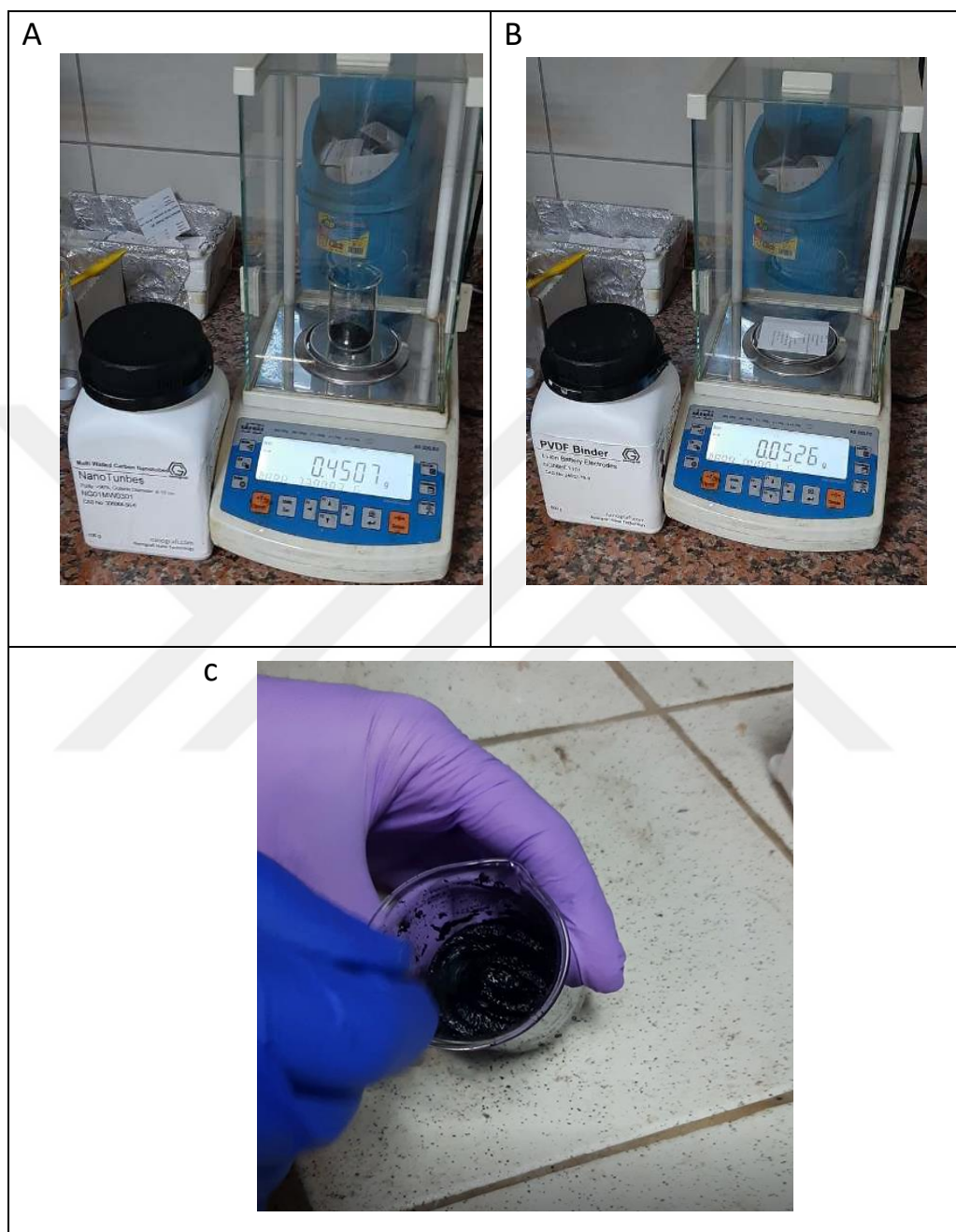
Figure 3.2. Photos of the procedure for preparing ink samples; A: CNTs weighing process, B: PVDF weighing process, C: The consistency of the final ink
