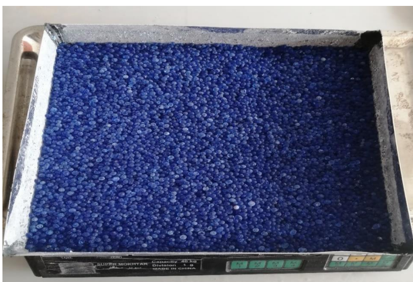
Figure 3.22. Silica gel after the drying process
