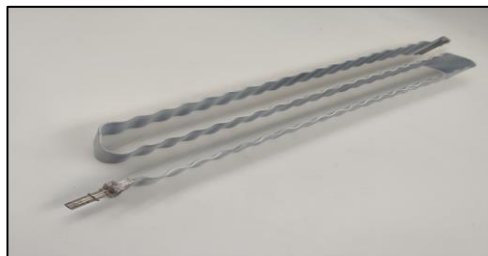
Figure 1.3: Serpentine Channels Cooling Plates.[9]
