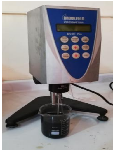
Figure 3.16: Photographs of Viscosity Measurement.
