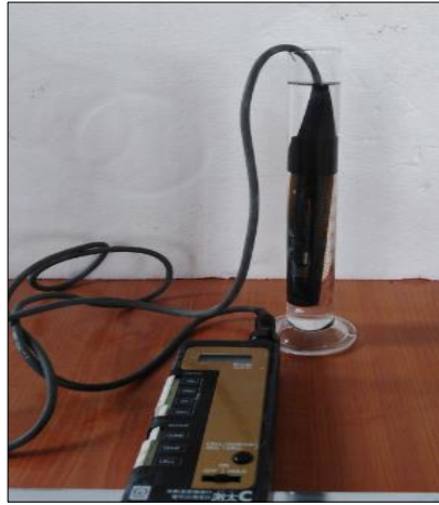
Figure 3.15: Photographs of Measuring Thermal Conductivity.
