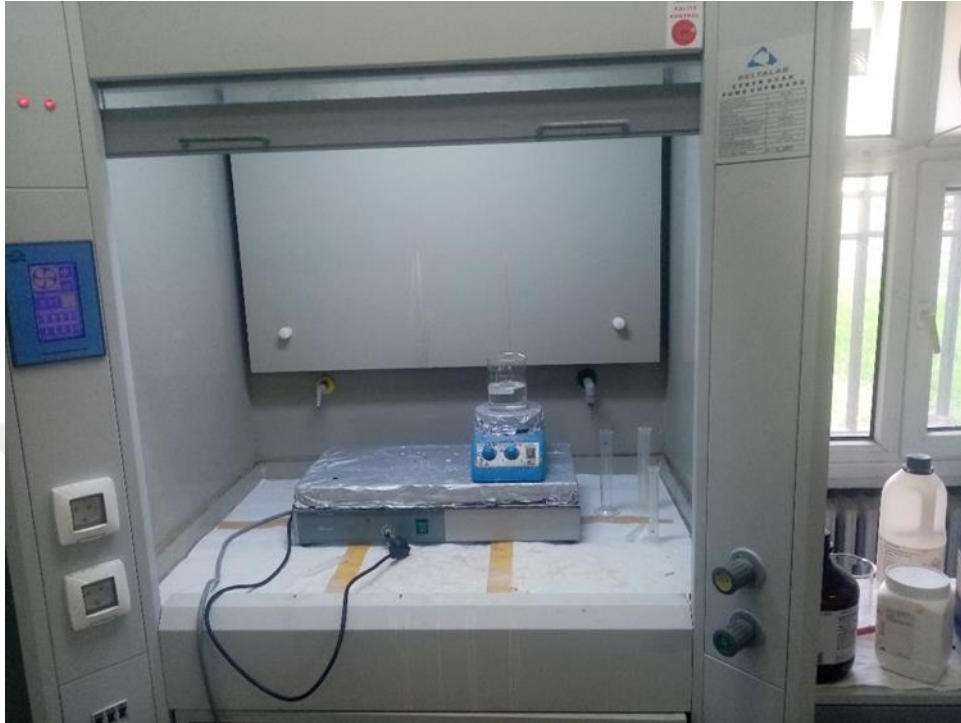
Figure 3.23. Preparation of the alkaline activator of NaOH and \text{Na}_2\text{SiO}_3
