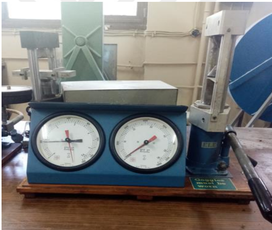
Figure 3.20. Point load strength measuring device
