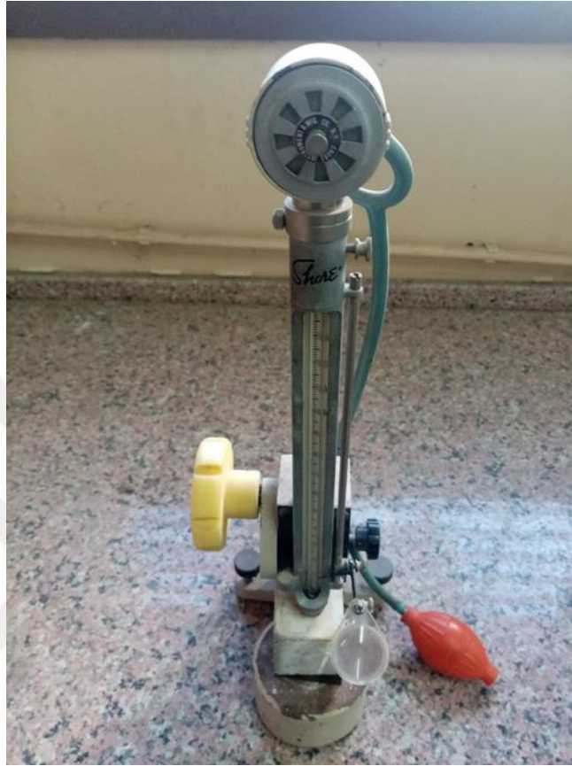
Figure 3.22. Device for measuring shore hardness
