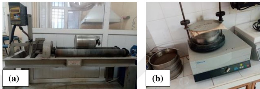
Figure 3.11. (a) ball mill rotator used in experiments, (b) retsch sieve Shaker AS 200 used in experiments.
