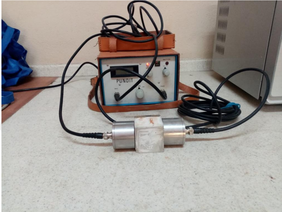
Figure 3.21. Pundit sonic speed tester used in the experiments.
