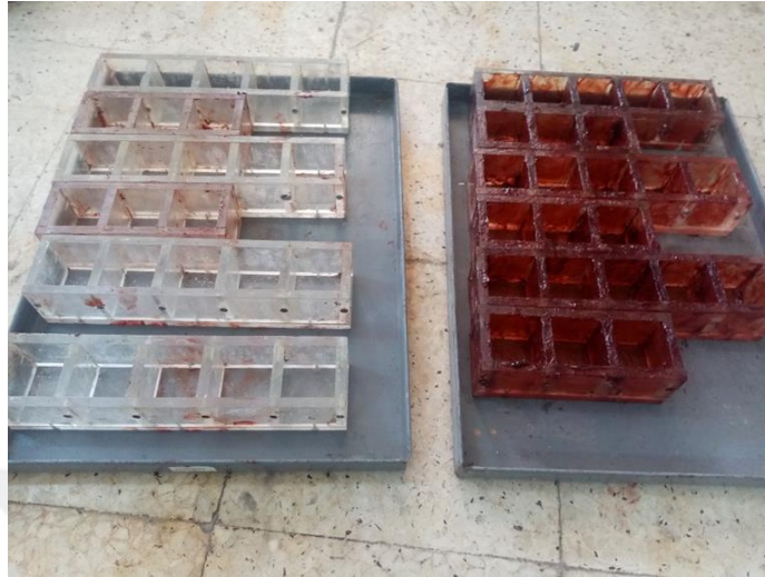
Figure 3.24. Geopolymer concrete casting molds
