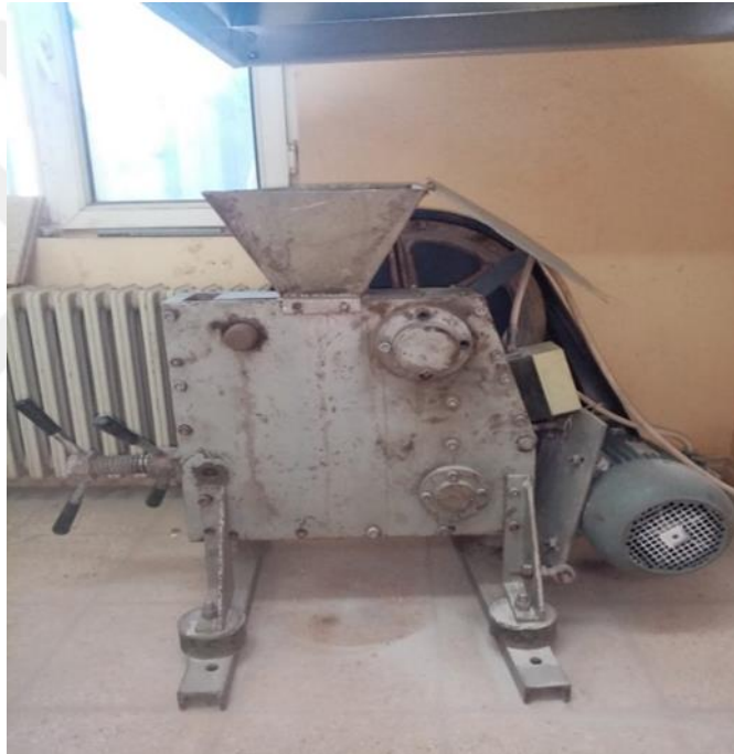
Figure 3.10. Jaw crusher used in experiments.
