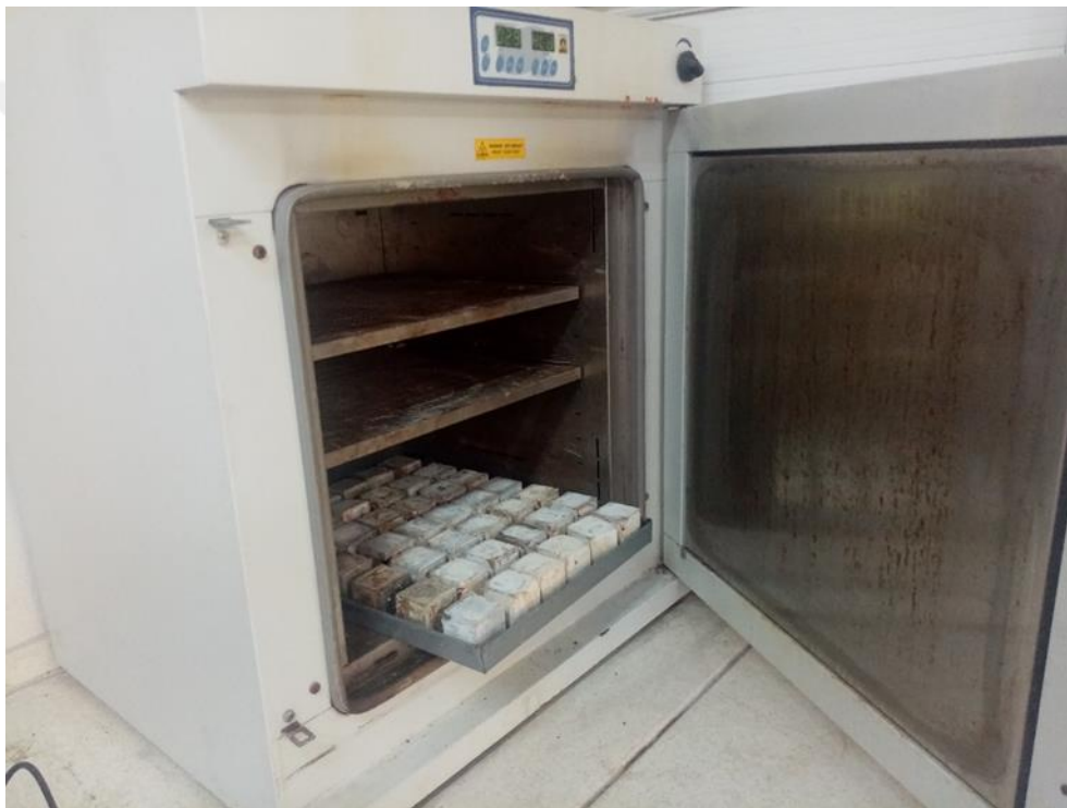
Figure 4.8. Heat curing furnace for geopolymer concrete samples
