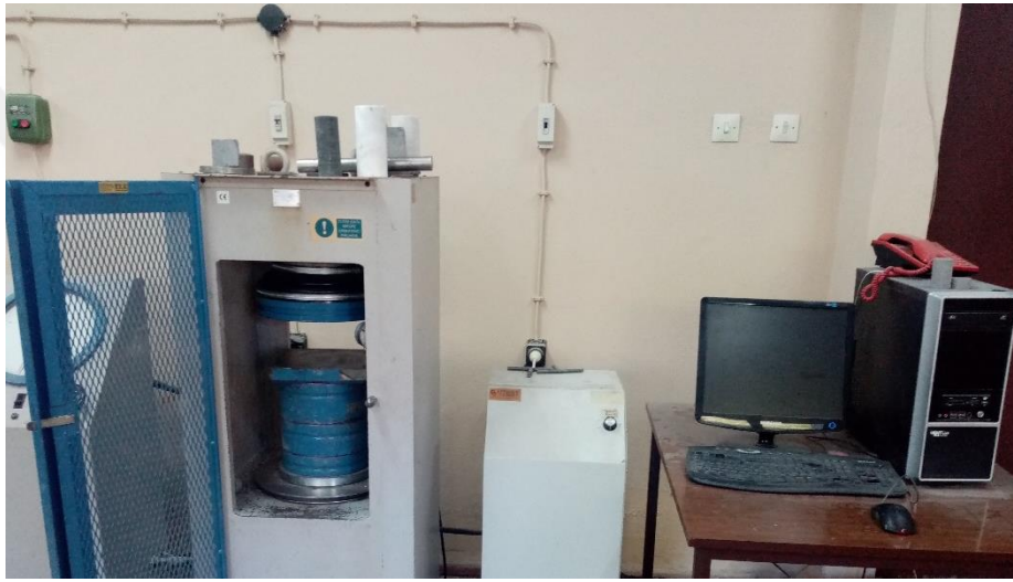
Figure 3.19. Device for determining uniaxial compressive strength.
