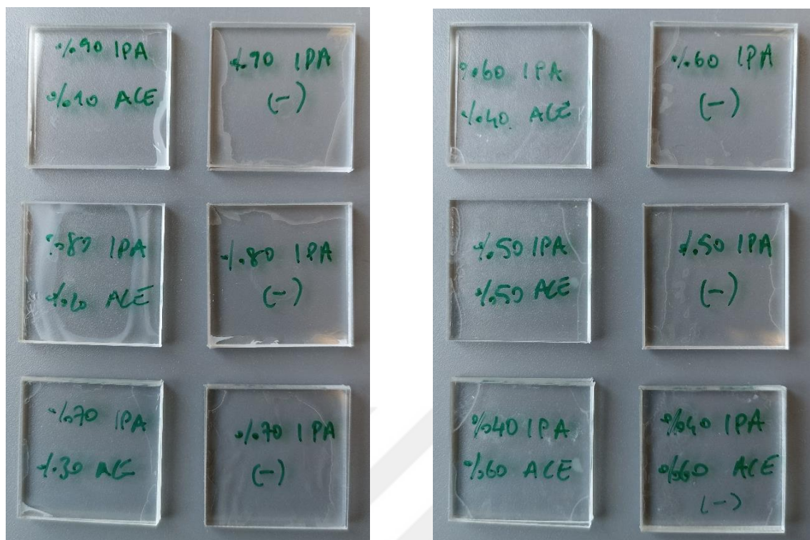
Figure 3.7: Bonding coverage image of PMMAs with different concentrations of isopropyl alcohol and acetone. The right part was bonded without plasma treatment.
