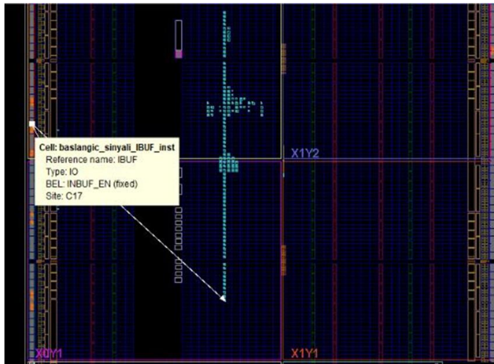
Image 5.7. The start signal and its route to trigger carry delay line
