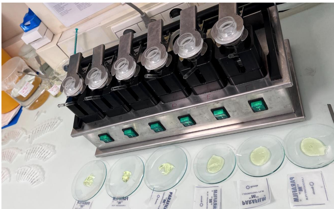
Figure10. Preparation of the Permeation Experiments with Franz Diffusion Cell Apparatus Used in the Lab for This Study.
