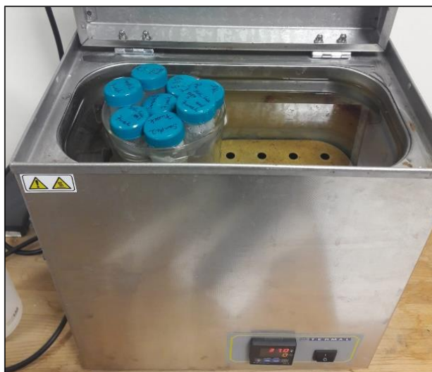
Figure 2.10. Water bath which was used for immersion tests.
