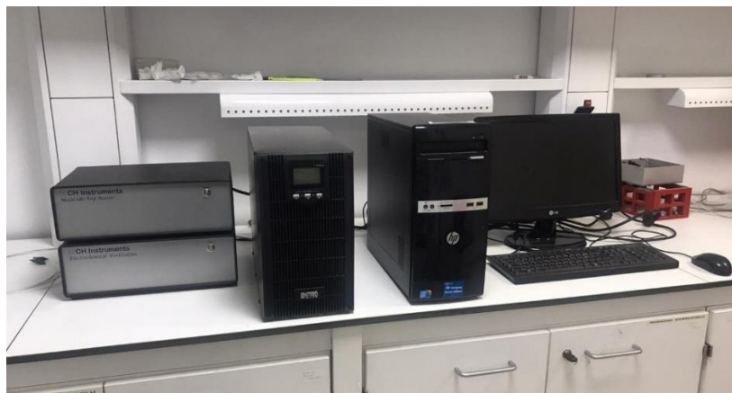
Figure 3.7 Corrosion resistance test equipment including Ch Instruments Electrochemical workstation device.
