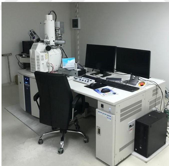
Figure 3.5 HITACHI SU5000 Field Emission Scanning Electron Microscope (FE-SEM) with the Energy Dispersive Spectroscopy (EDS) detector.
