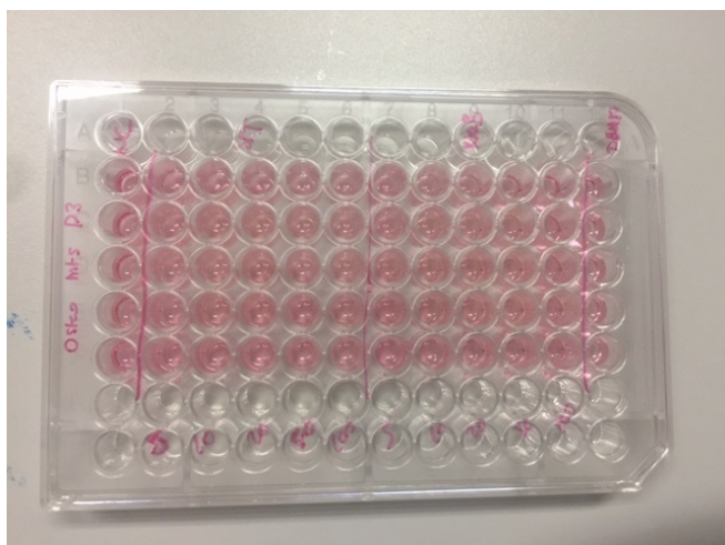
Figure 3.10 Placement of TiB 2 extracts and control medium into wells with SaOs-2 cell line
