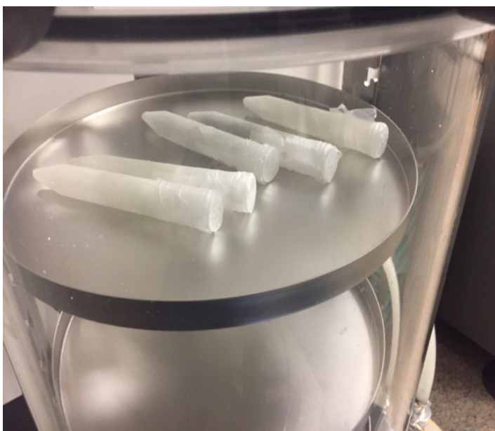
Figure 3.3 Lyophilization of chitosan scaffolds.
