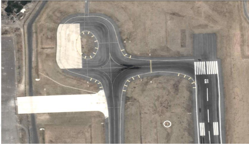
Şekil 2.8. Döngüsel taksi yolu (loop taxiway) (aviation.stackexchange.com,2018)
