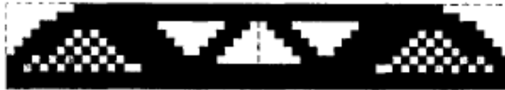
Figure 2.4: Checkerboard patterns on optimized structure.
