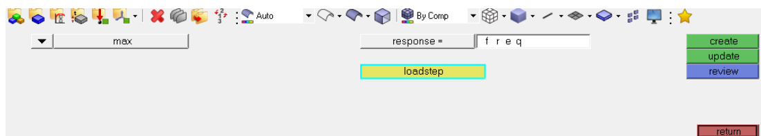
Figure 5.13: HyperMesh screenshot to create load step.
