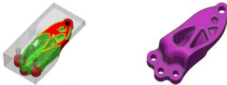
Figure 1.4: Optimization output and optimization based CAD model.
