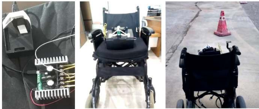
Figure 5.4 The PWC used during experiments and development with the installed hardware (battery, Raspberry Pi, motor controller and camera).
