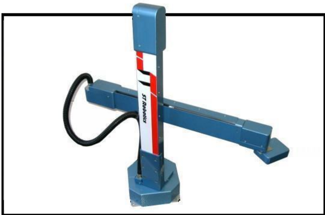
Figure 2.2 Cylindrical robot (R19 ATHENA series, ST ROBOTICS)
