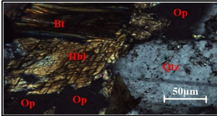
Figure 4.47. shows the crushed margin of amphibole with chlorite due to alteration and associated with opaque minerals. Hbl- Hornblende, Bt- Biotite, Op- Opaque mineral, Qtz- Quartz. (Sample- AM22).
