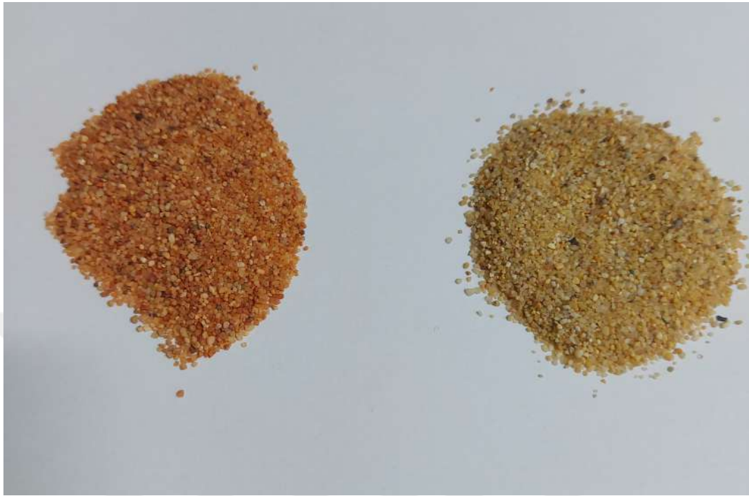
Figure 4.2: Comparison of cycled (left) vs non-cycled (right) sand particles
