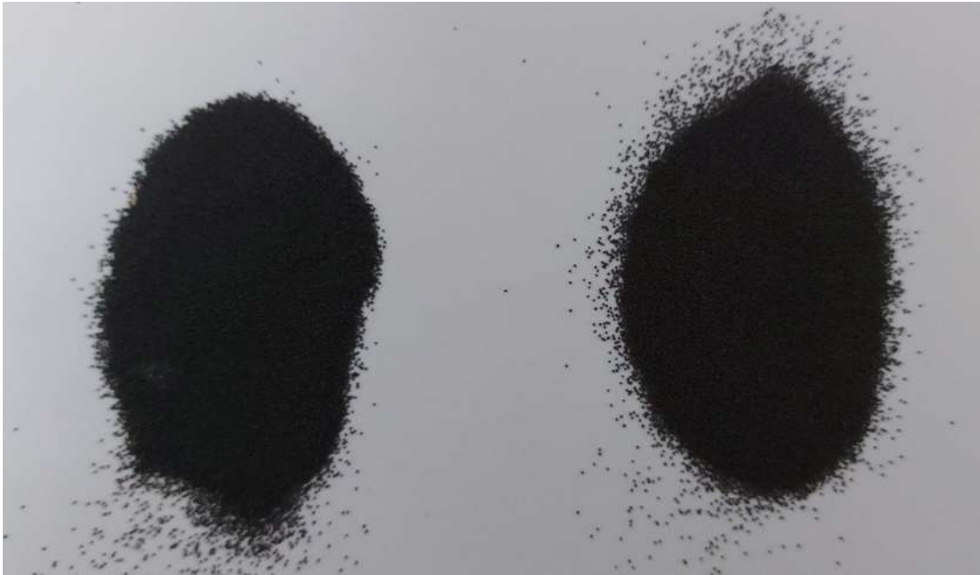
Figure 4.1: Comparison of non-cycled (left) vs cycled (right) CarboHSP 40/70 particles
