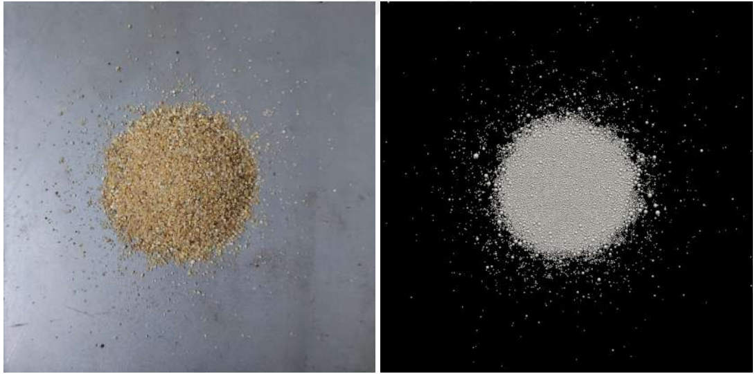
Figure 3.28: Particle scattering comparison of test (left) and DEM model (right) for sand
