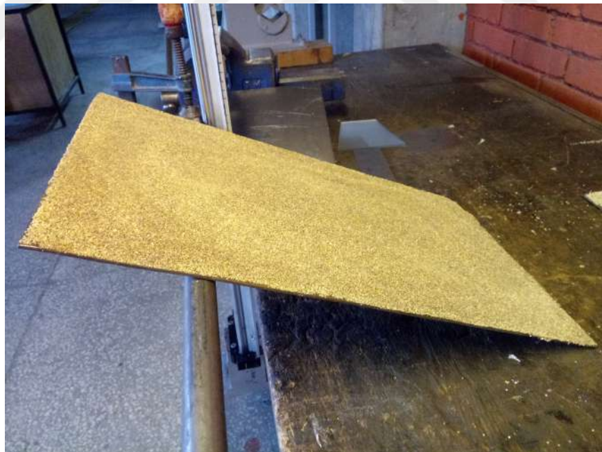
Figure 3.5: Inclined plate test setup
