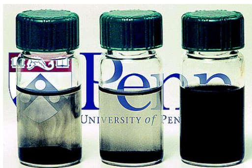
Figure 3.4: Photograph of poorly dispersed SWCNT solutions (2 images on left) and a well dispersed SWCNT solution (image on right) [65].
