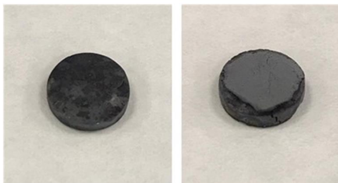
Figure 6.10 Deformation of the samples after thermal diffusivity measurements.
