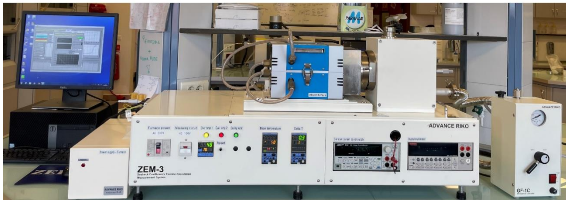
Figure 3.8 Ulvac Zem-3 electrical resistivity and Seebeck measurement system.
