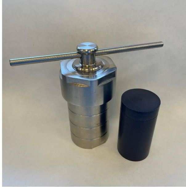
Figure 3.4. Hydrothermal stainless-steel (316 L) autoclave reactor and polypropiolactone (PPL) liner.
