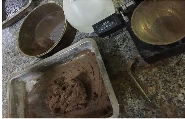
Figure 3.11 Determination of atterberg limits in laboratory.
