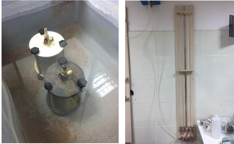
Figure 3.13 Falling head permeability test in laboratory.
