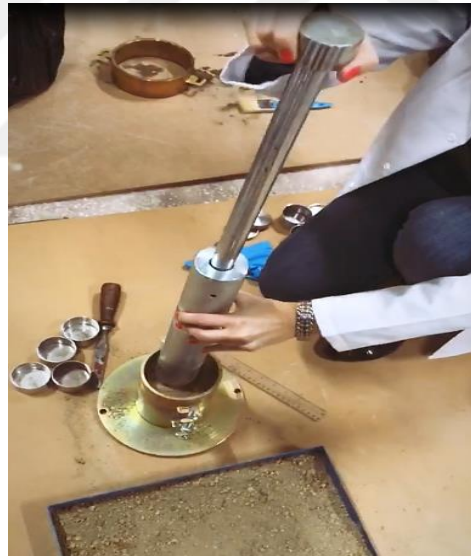
Figure 3.12 Standard compaction test in laboratory.
