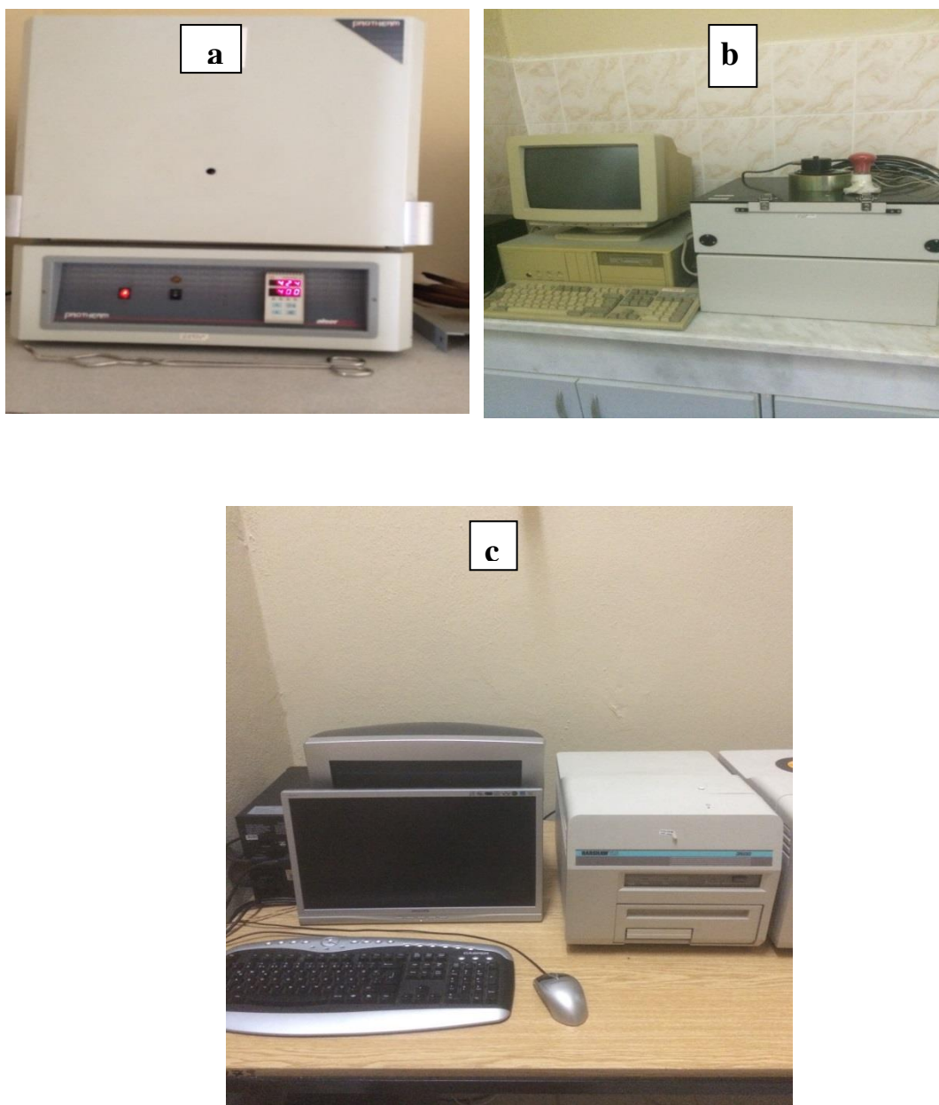
Figure 4.1 (a) the oven, (b) irradiation part, (c) TLD reader
