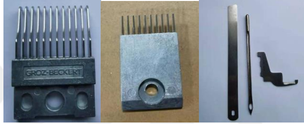
Şekil 3.8. Tufting Halı Makinesi İğne Ekipmanları ( http://carpet-machinery.web.tr/4-carpet-tufting-machine.html 27.09.2024)
