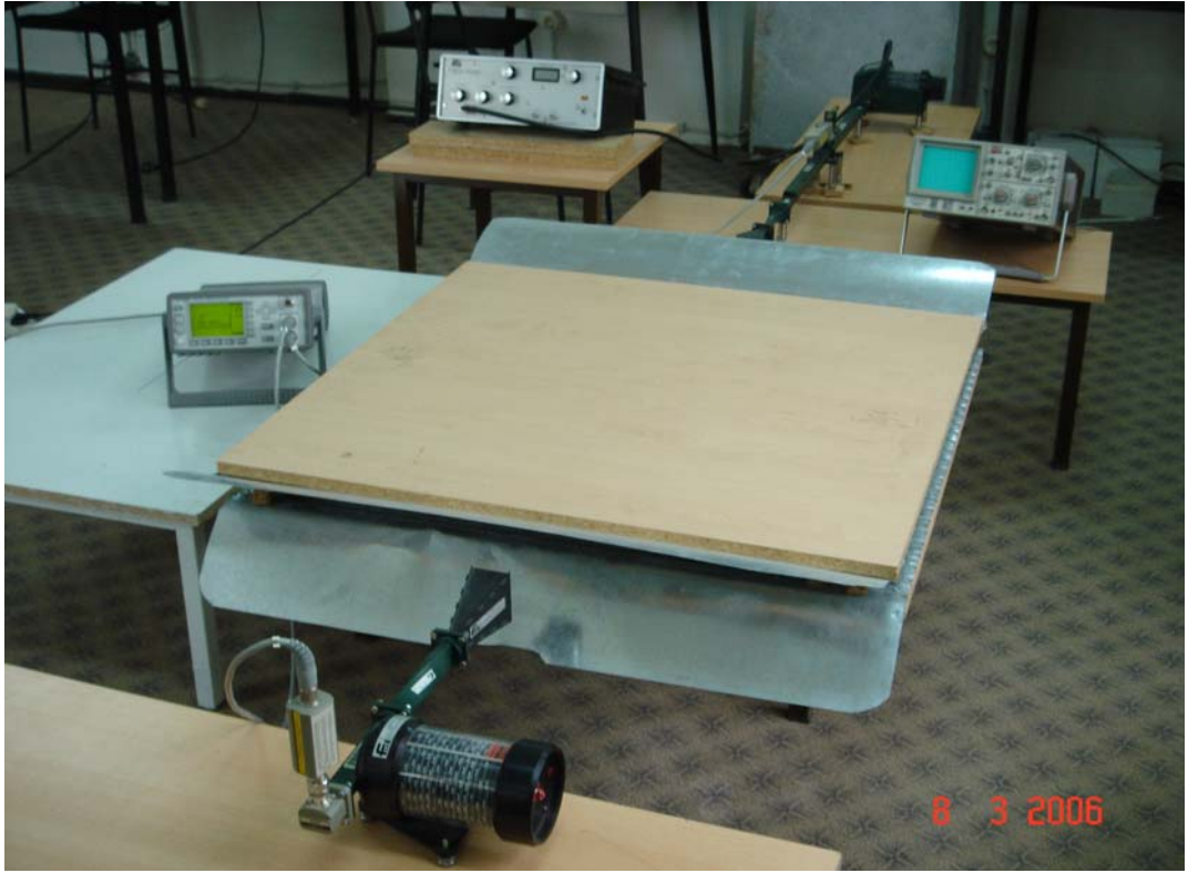
Fig. 3.4. Experimental setup. It consists of oscillator, two couplers, Agilent E44196 power meter and two X-band pyramidal horn antennas. Flares were placed at the edges of the waveguide facing the receiving and transmitting antennas in order to minimize reflections of the guided electromagnetic wave from edges.
