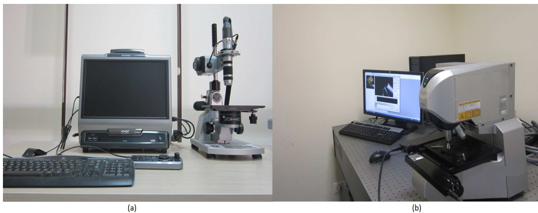
Figure 3.2 General views both VHX-1000 digital and VK-X100 3D laser scanning microscopes.
