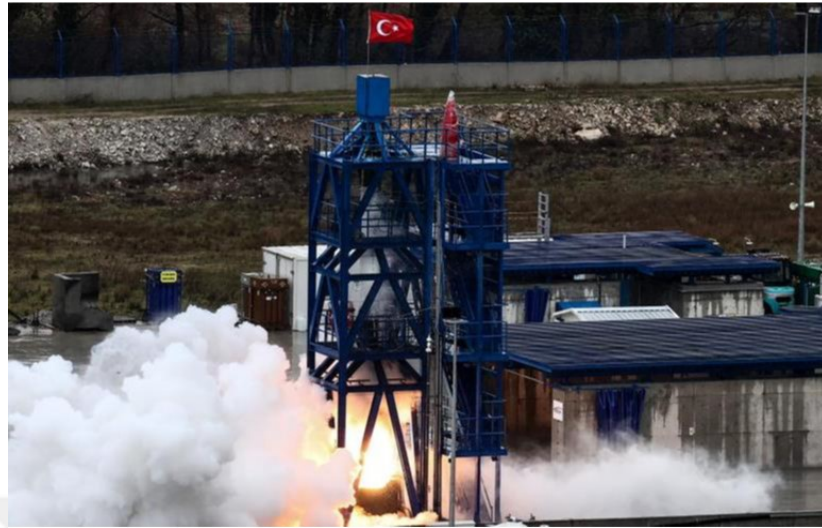
Figure 1.6. Image from DeltaV Space Technologies' static firing test [7].
