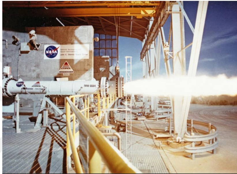
Figure 1.5. Image from AMROC H-1800 hybrid rocket test [6].
