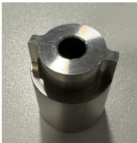
Figure 3.8. Coupling used in RPM sensor tests.
