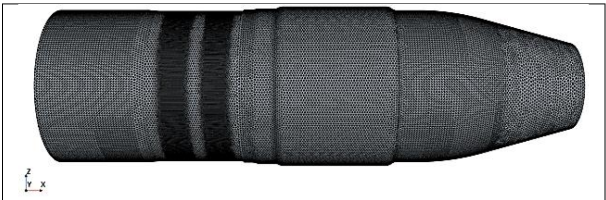
Figure 4.5: The meshing procedure implemented to the whole jet engine.
