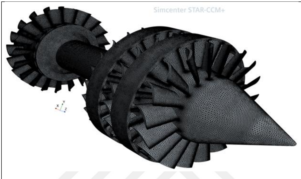
Figure 4.6: Meshing process applied to the inner parts of the jet engine.
