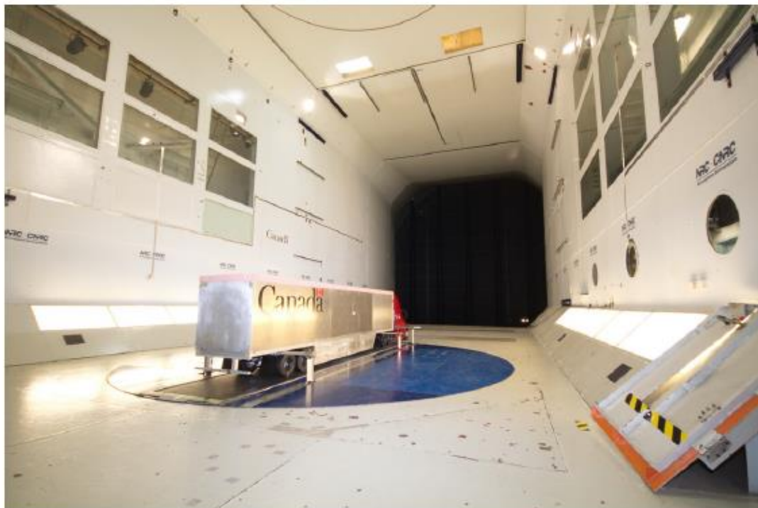
Figure 2.31: The tractor-trailer model investigated in the Canadian Wind Tunnel with a total length of 9 m [57].
