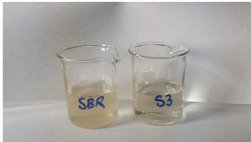
Figure 4.52 SBR effluent (L) – SBR+MBTF+S3 Effluent (R) (Personal archive, 2020)
