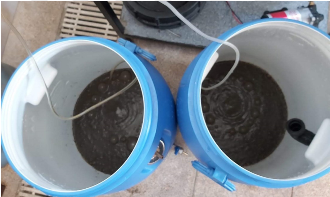
Figure 3.4 Activated sludge tank and SBR (Personal archive, 2019)
