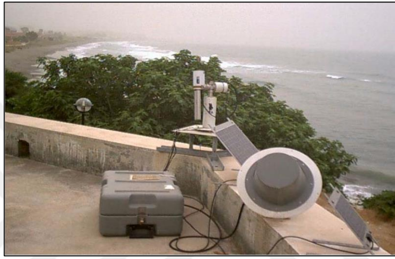
Figure 2.8 CIMEL Sun-photometer (Kubilay & Koçak, 2009)
