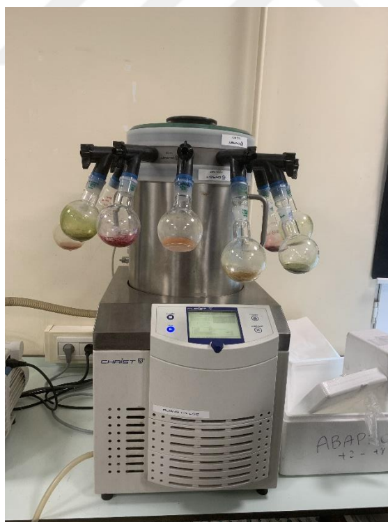
Figure 10. Lyophilization process of Crataegus extracts.
