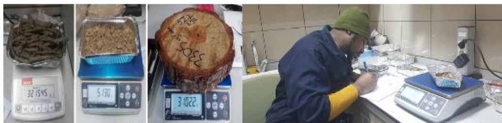
Figure 49. Weighing of samples before and after oven-drying
