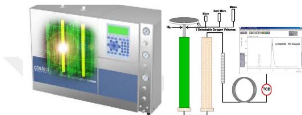
Figure 54. Combustion and detection process in the COSTECH Analyzer
