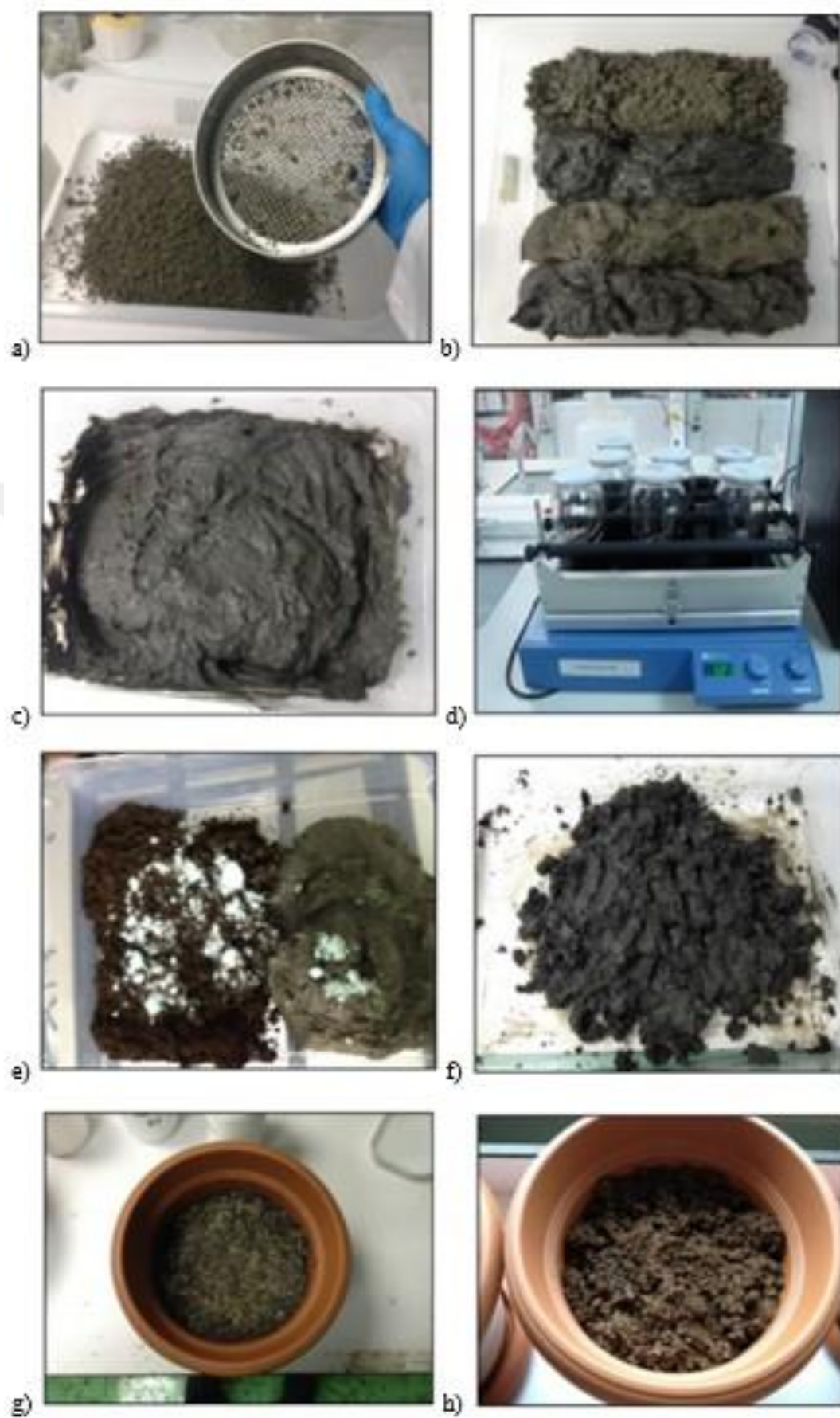
Figure 4.2. Preparation stages of MT samples
