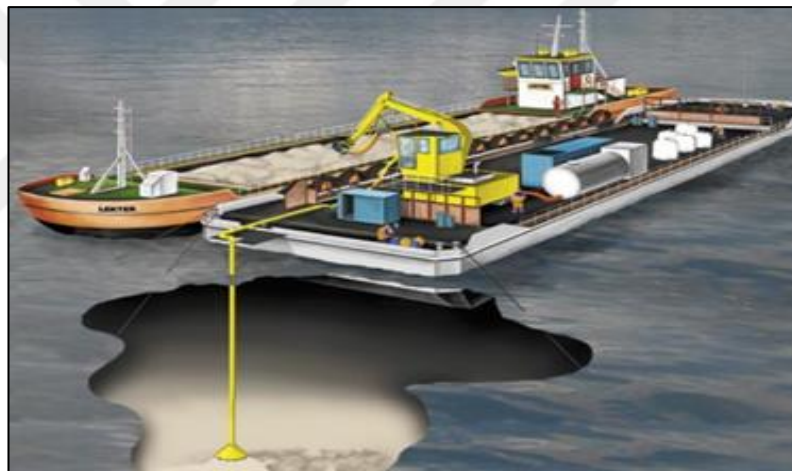
Figure 1.1. Typical dredging equipment at the middle of the sea or lake (Pettersen et al., 2007)
