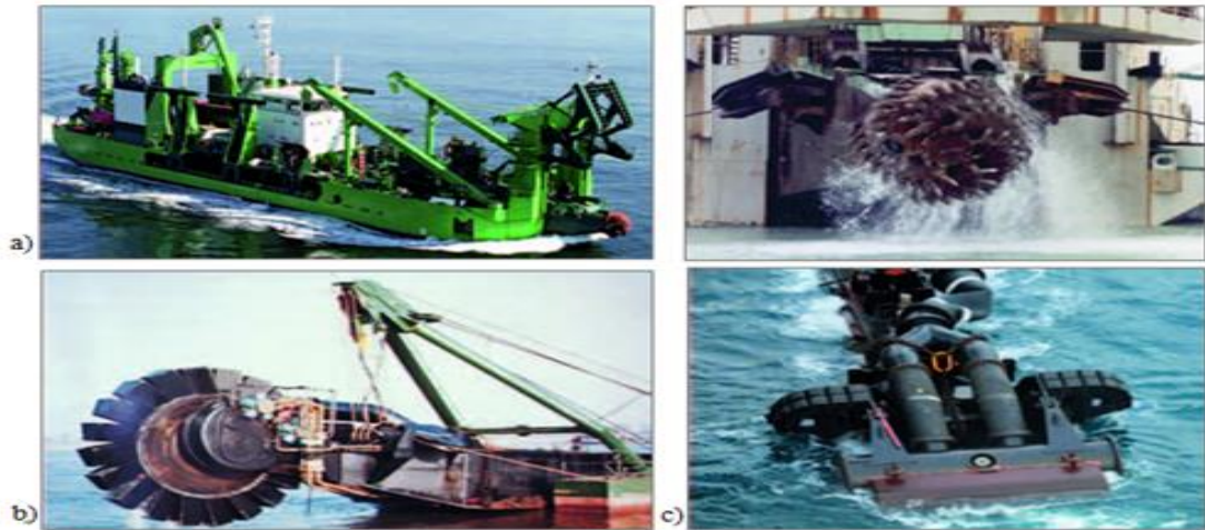
Figure 1.6. Mechanical/Hydraulic dredgers; a) cutter suction or cutter-head dredger, b) bucket-wheel dredger, and c) trailing suction hopper dredger (Bray and Cohen, 2010)
