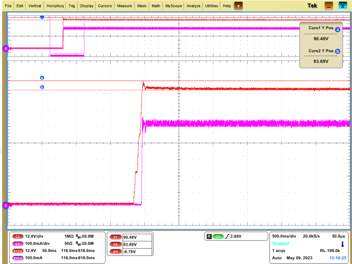
Figure 34 Measured LED output voltage and current at start-up
