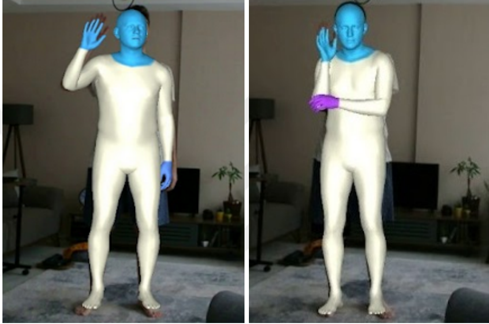
Figure 2.2: Example reconstructions using PIXIE, without using the FLAME [3] model. On the right, the elbow rests on the actor’s hand and causes occlusions. Such occlusions lower the confidence of reconstruction.
