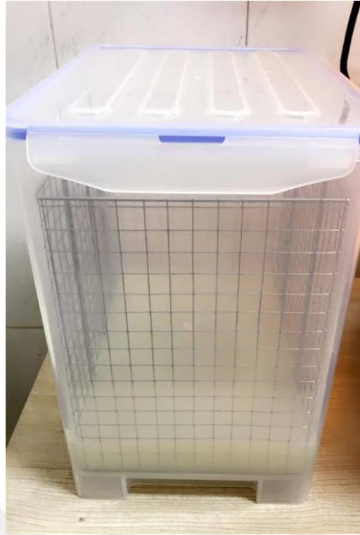
Figure 3.2.3.2.B. Washing Container contain 91% isopropyl alcohol
