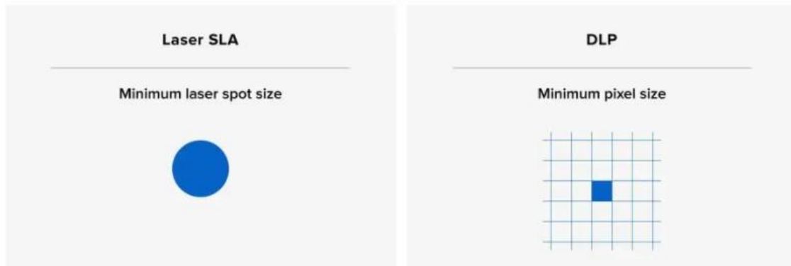
Figure 5.2.4. Difference in the shape of the basic core element between SLA and DLP printers.(207)
