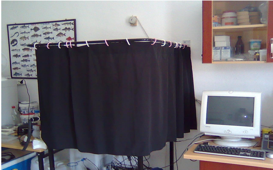
Figure 3.6. The tank of the respirometry was covered by black curtain to prevent burst activity during the experimental period.
