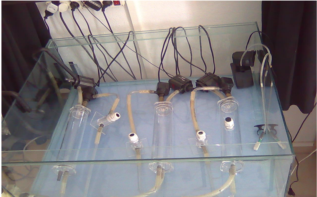
Figure 3.4. Structure of respirometry tank with three chambers.
