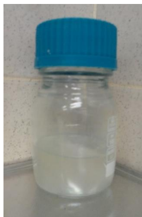
Figure 4.8: 13 wt% TPU as electrospinning solution.
