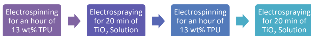
Figure 4.12: Schematic of fabrication of sandwich structure.
