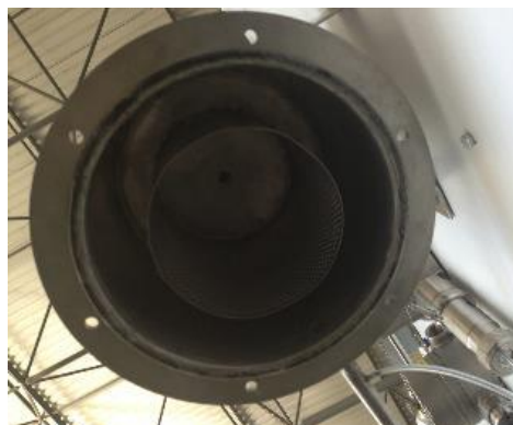
Figure 5.7: Support for nanofibrous filter.
