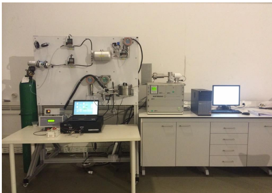
Figure 5.4: 2 nd generation UV-LED system built with an in-situ VOC generation and detection system.
