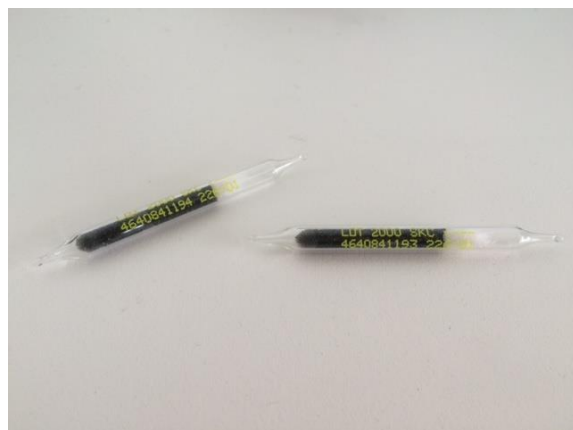
Figure 5.3: Active carbon sorbent tubes for sampling.
