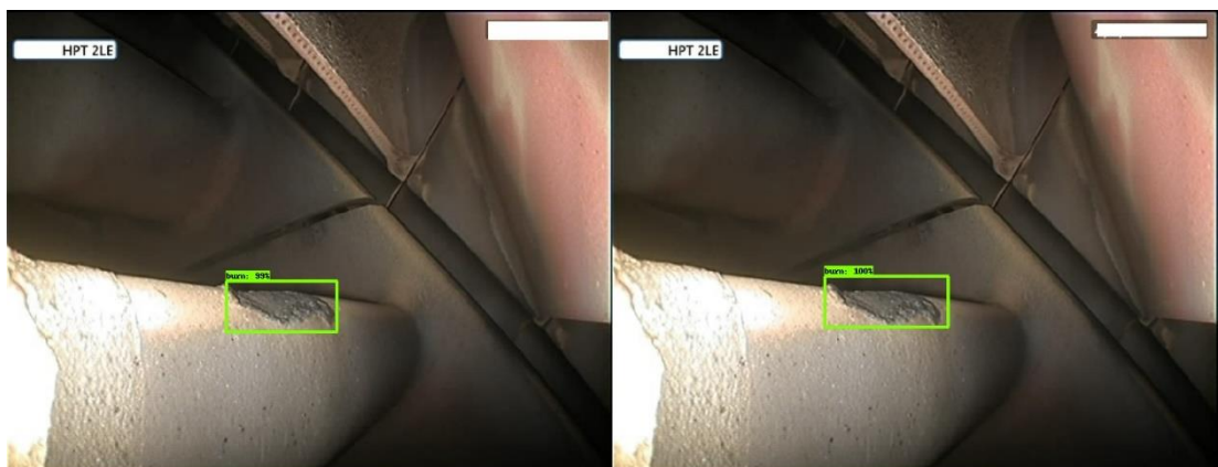
(c) Burn detection sample. Right image the ground truth, left image the detection
