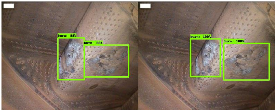
(c) Multiple burn detection sample. Right image the ground truth, left image the detection
