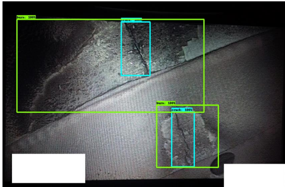
(e) Multiple burn and cracks with overlapping areas as well as huge burn with no natural boundaries
