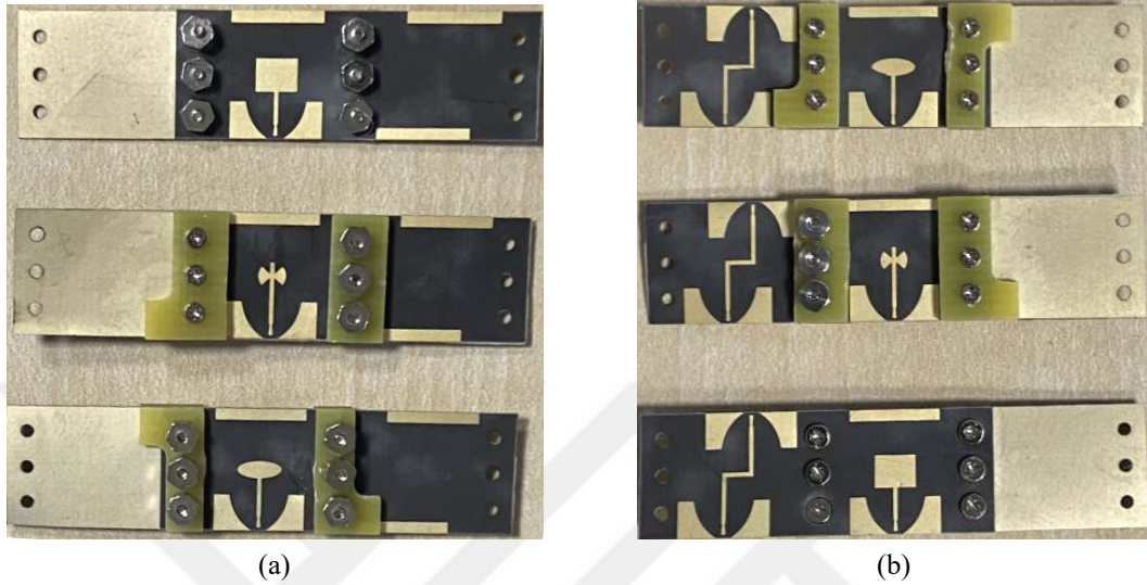
Figure 3.8: (a) Front view of the coupler with the butterfly shaped resonators. (b) Back view of the coupler with the butterfly shaped resonators.
