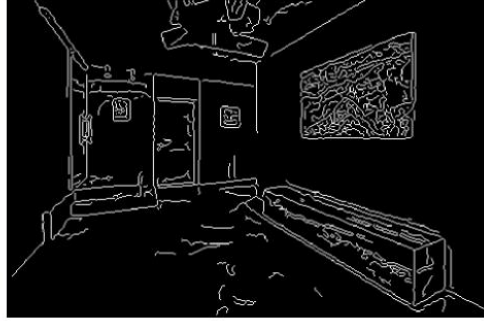
(a) Wireframe image (Huang et al., 2018) (b) The Canny edge detector ( [0.05, 0.1], 1.2 ).
