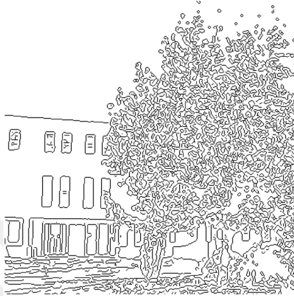
Figure 1.8 The result of the Canny edge detector ([0.05,0.1],1.2).
