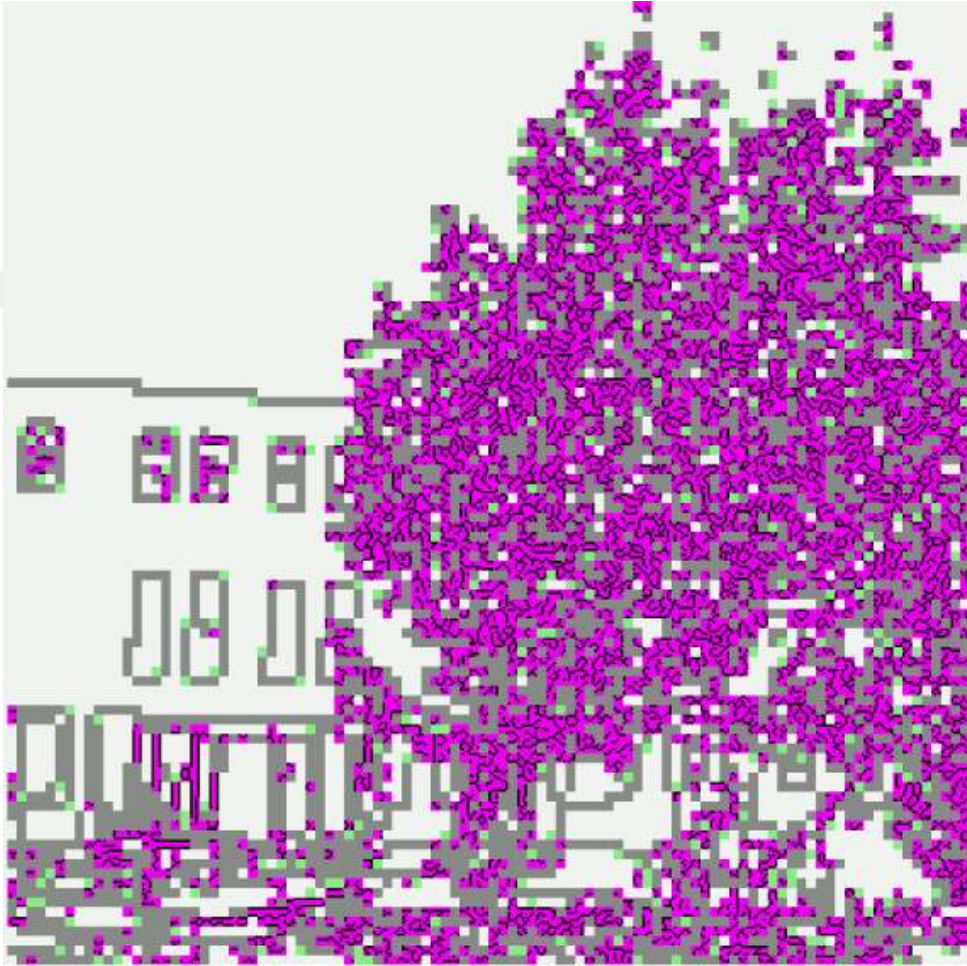
Figure 3.11 The unrecognized 4 \times 4 pixel edge patterns are painted in pink and eliminated.
