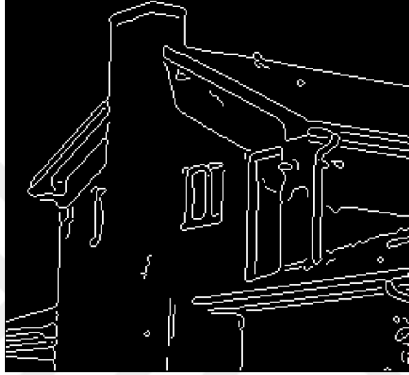
Figure 3.7 The result of Canny ([0.05,0.1],1.2) edge detection for the House image.
